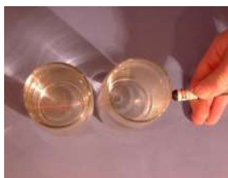
Fig. 3 The laser beam is visible as it crosses the second glass (colloid) but not the first one (water).
