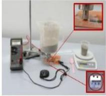
You can use either lab masses or a beaker progressively filled with sand (add a constant quantity each time). At first, when the exerted pressure is still low, the QTC resistance will fluctuate and reach a fixed value only after a while. This is why, when adding a new mass, it's extremely important to have all the readings after the same time has lapsed (say 0,5 or 1 sec). Repeat the experiment with different conductive polymers (such as Velostat or Eontex) and compare results.
