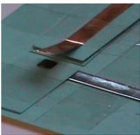
To connect the QTC pill into the circuit, put it between two thin metal strips (“embossing copper” sheets used at school in arts and crafts work fine. QTC should be in contact with the silvery side!). Fix them with tape directly on the table or any other stiff electrically insulating surface (cardboard is ok too). Careful! The two strips must not be touching in any way: Current should flow from one to the other only through QTC !
