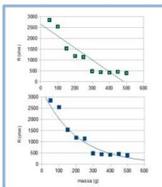
Once you have collected data, search for the theoretical model that fits the resistance VS pressure relationship best. Repeat the procedure for each sample and compare results. You can make use of the best-fit curves functionality in the electronic sheet and of specific control tables.
