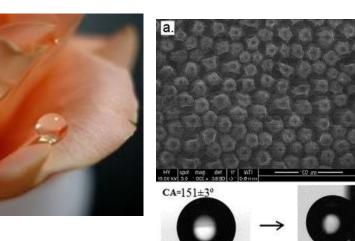
Fig. 9 Drops on rose petals show an incredibly high contact angle and at the same time an extremely strong adhesion. Image courtesy M Karaman Department of Chemical Engineering, Selcuk University, Konya, Turkey.
