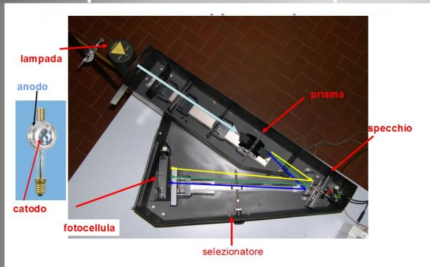
Experimenting with photoelectric effect students are led to understand some basics of Quantum Mechanics such as light and matter interaction, energy quantization, Planck's constant.
